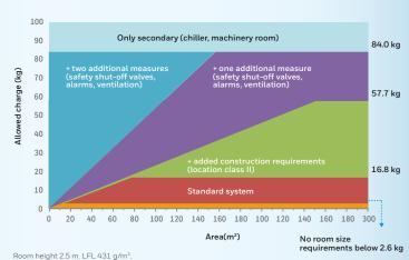
Examples of how charges are calculated depending on the application according to the EN378 standard
